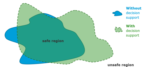
Figure 2. Illustration of the safe and unsafe regions for a ship navigating with and without functionality for autonomous navigation and decision support.
