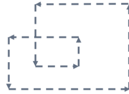
Figure 3: Example of a loop with 720 degrees turns before returning to the start
